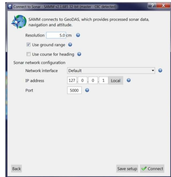
Figure 56. SAMM Interface to GeoDAS
